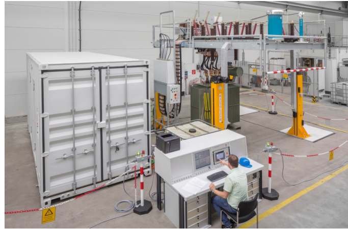
Diagram 8. Shop test of a DiTAS at HIGHVOLT using a platform lift before customer delivery
